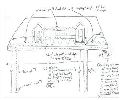
Roof & Gutter Deicing Sketch Installation Planning
